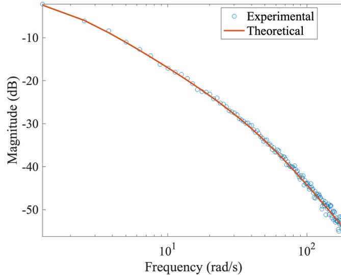
**Figure 9:** The closed loop bode plot describing the voltage-position relationship of the motor. The bode plot of the theoretical closed loop transfer function is provided based on the estimates of  $\tau$  and  $K$  from the voltage-velocity model.
