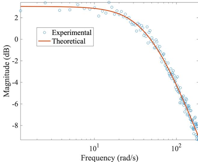
**Figure 7:** The experimental bode plot of the voltage-velocity relationship obtained from 150 superimposed sine waves.
