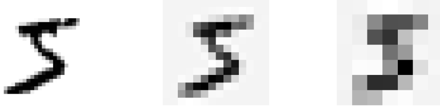
Figure 4: The bicubic interpolation to reduce the size of the image. (left) Original, (center) scaled by 0.25, (right) scaled by 0.0625. The image is the first element of the mnist dataset.
