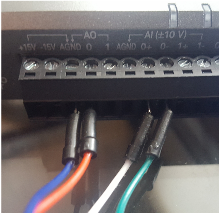
Figure 5: The wiring diagram of the myRIO for proportional control of an RRC circuit, using analog input and output.
