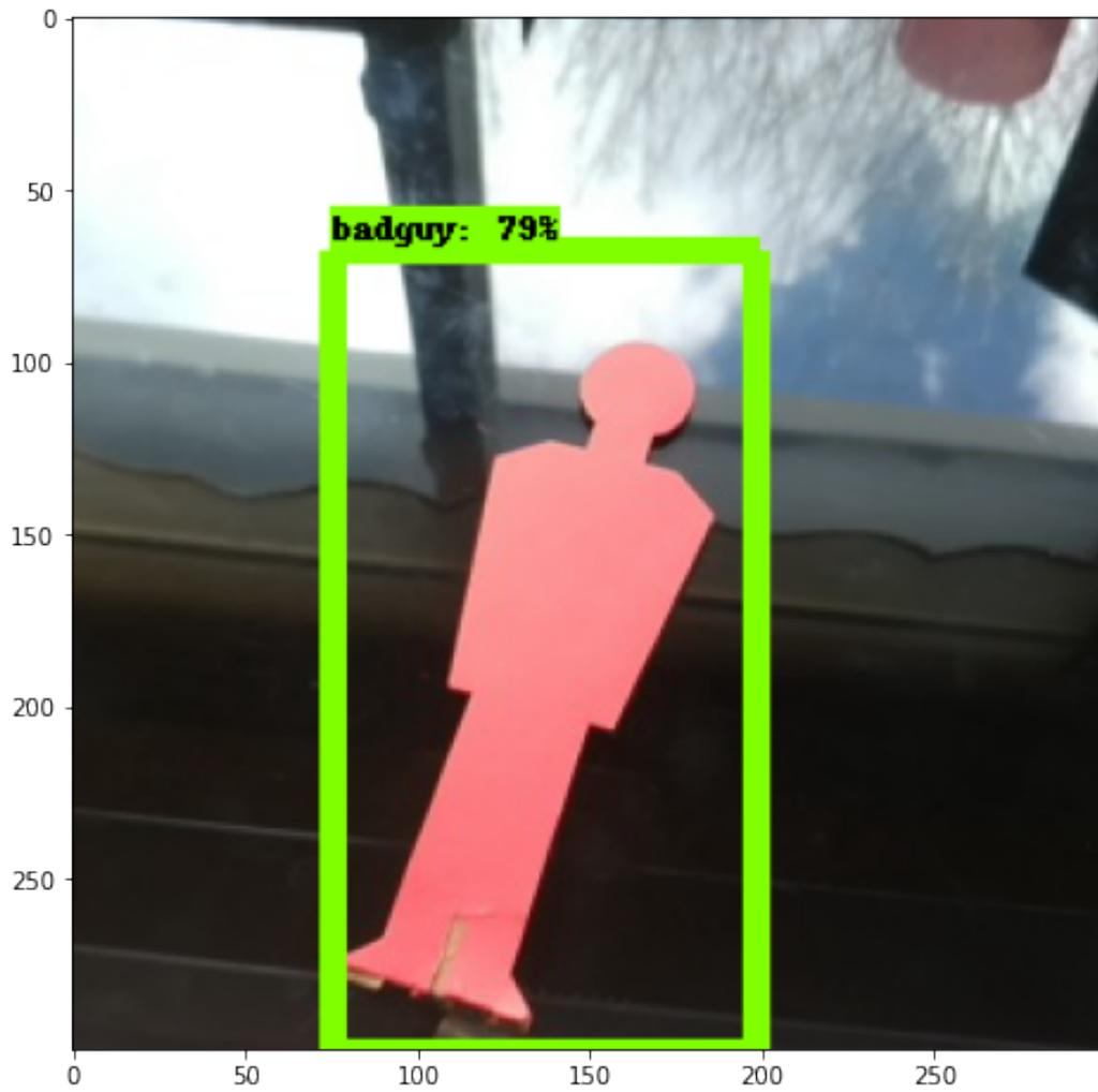
**Fig. 1** The target was identified with a probability of 79%, and drew a bounding box accordingly.
